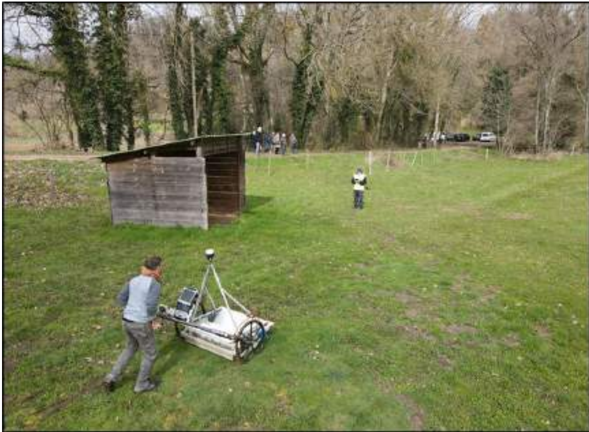
Figure 3: Le GPR en acquisition
